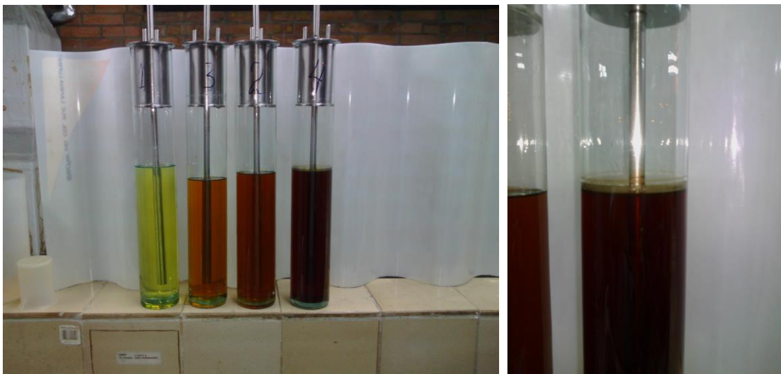
Fig.6. Mixtures image after the test. Note adherent Gum ring on top of Mixture No. 4
