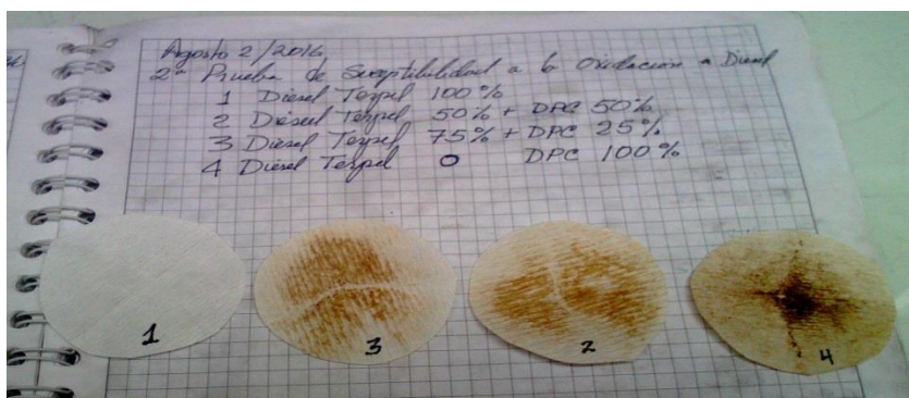
Fig. 9. Insoluble Gum formation in mixtures of Diesel Terpel and Diesel DPC.
